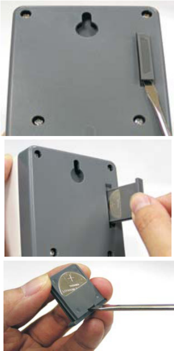
Fig. 06 - Instruction to replace the TM-6331's battery
